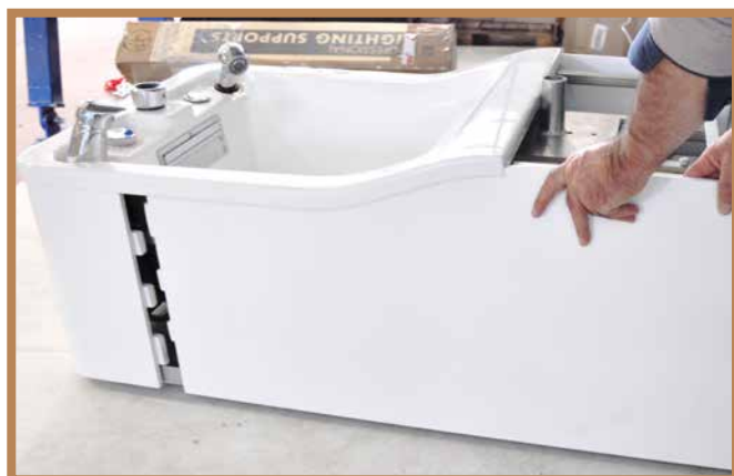
STEP 4: Remove the left lateral wooden cover.
